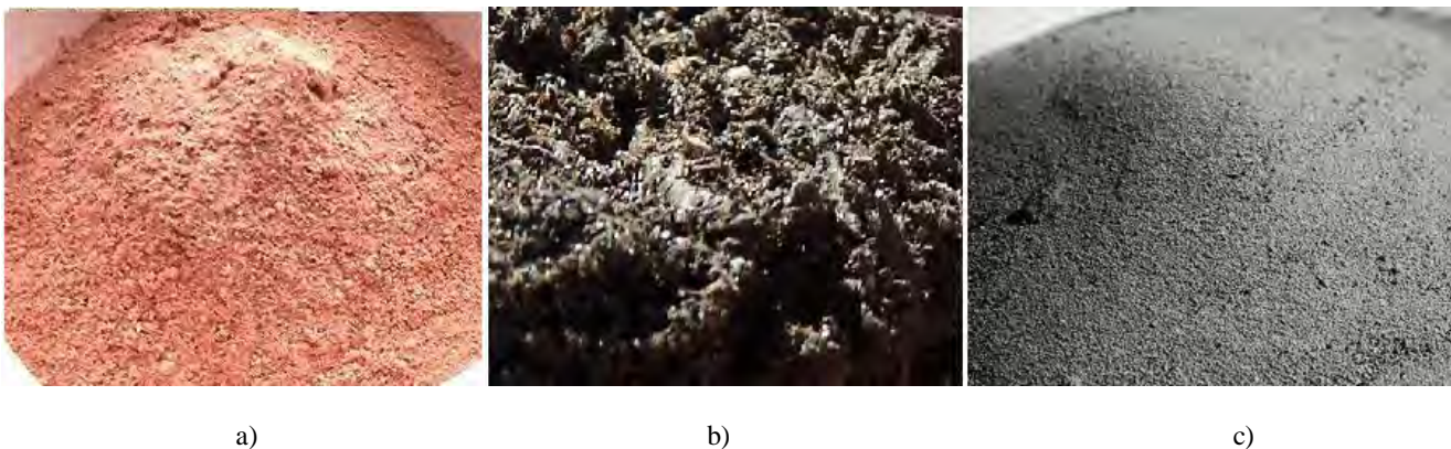
Fig. 4. The general view of man-made waste before and after processing with dispersers and methane fermentation: mixture of TPP water demineralization calcium sludge without processing (a); poultry manure without processing (b) and mixture of TPP calcium sludge, activated sludge, poultry manure after dispersion and methane fermentation (c)
