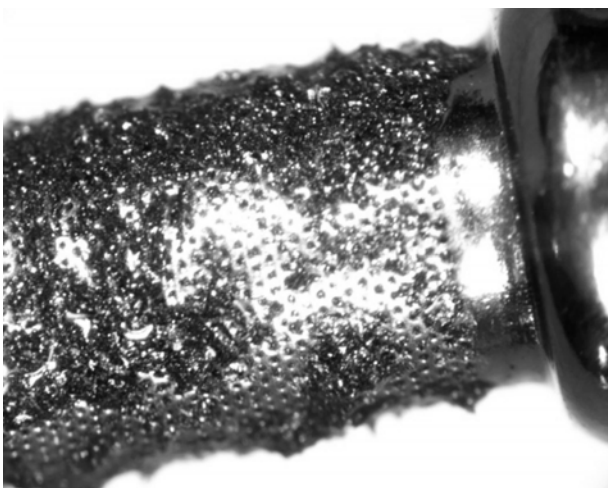
Fig. 4. Pressure regulator with visible metal filings shavings under a microscope
