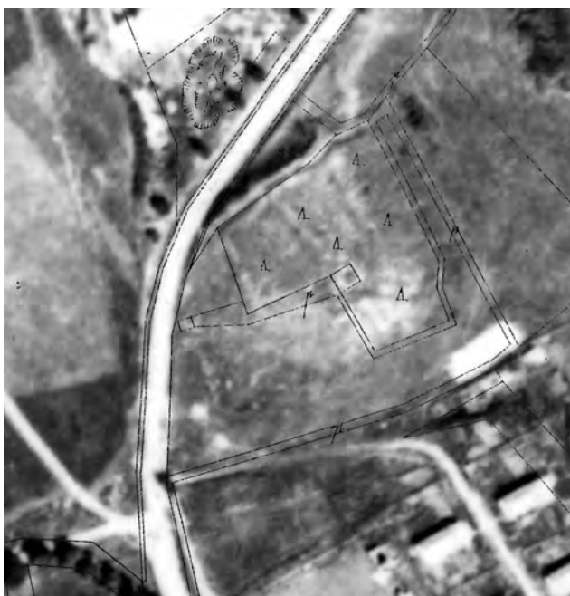
Fig. 6. Variant of synthesis of archival German aerial image with archival cadastral plan on the territory of Jewish cemetery in town Zhydachiv
