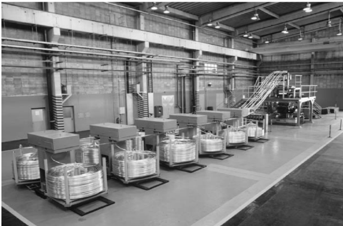
Fig. 2. Scheme of rolled copper production line by horizontal Continuous Casting Process
