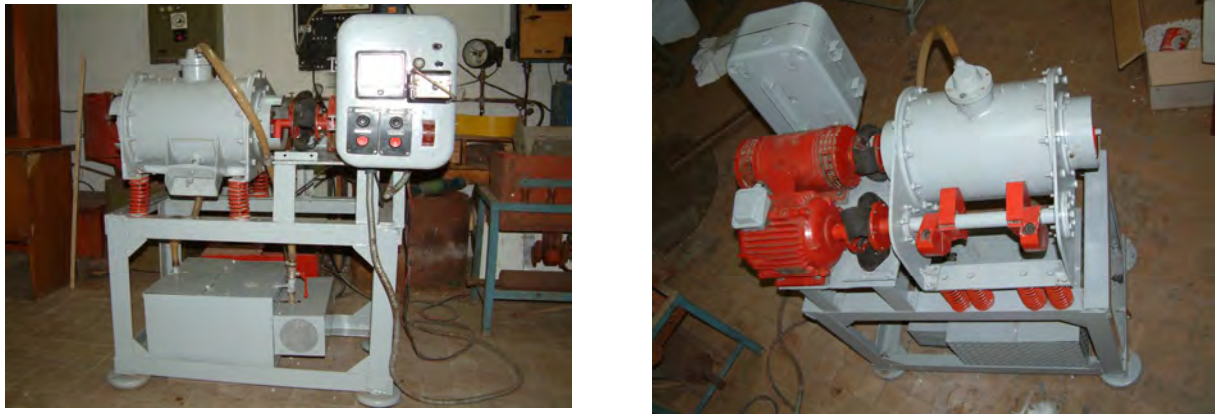
Fig. 2. A general view of machine for vibro abrasive treatment of the details
