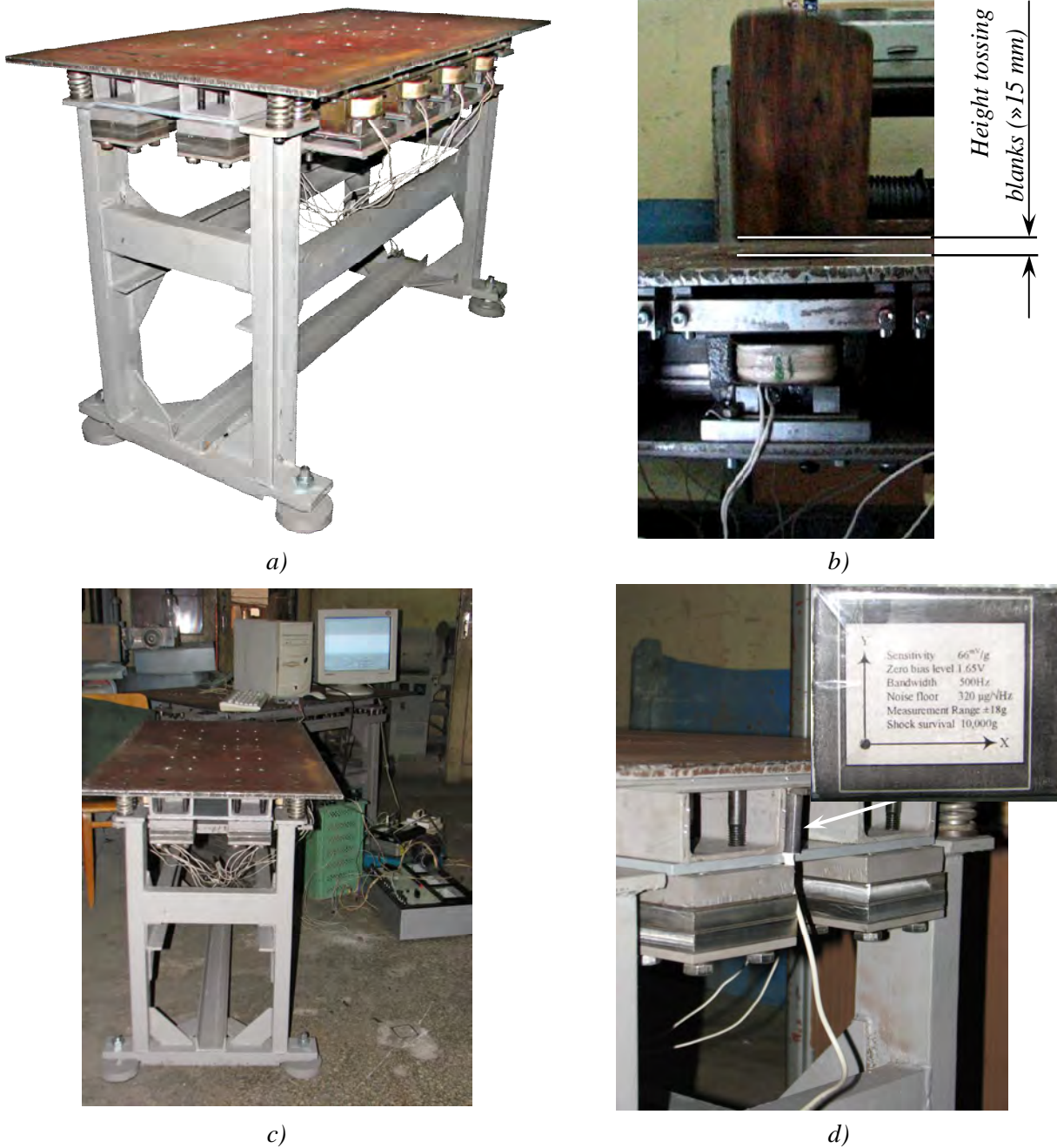
Fig. 23. Experimental sample of the vibratory table (a); fragment of video, where the work of the vibratory table is represented (b); arrangement of equipment during an experiment (c) and sensor which is connected to mass m_1 (d) for the output of time dependences of motion of oscillating mass
