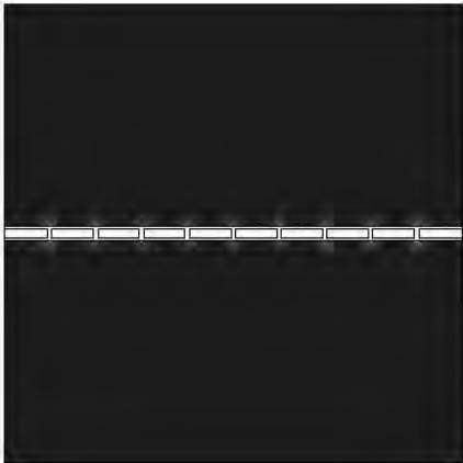
Fig. 9. Distributions of power volume density of the contact model with 9 equal contact surfaces
