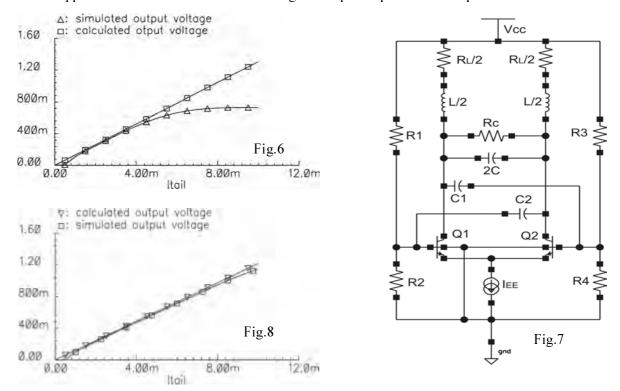
The results in this paper have been used to design 2.4GHz VCO for Bluetooth standard using 0.35um HBT BiCMOS technology of Austriamicrosystems. The VCO shows 800mV<sub>pp</sub> output amplitude, 2.38-2.68GHZ tuning range, phase noise 123dBc/Hz at 1MHz offset from the carrier, 26mW power consumption. (See "Fully-Integrated VCO with low phase noise", Nachev R., Ivanov K. and etc., Proceedings of the International Scientific and Applied Science Conference ELECTRONICS 2004).
