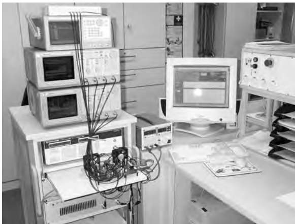
Fig. 23. Test set-up for DPI-measuring method
