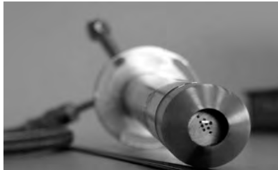
Fig. 2. Multichannel, measuring probe intended for use inside a combustion chamber
