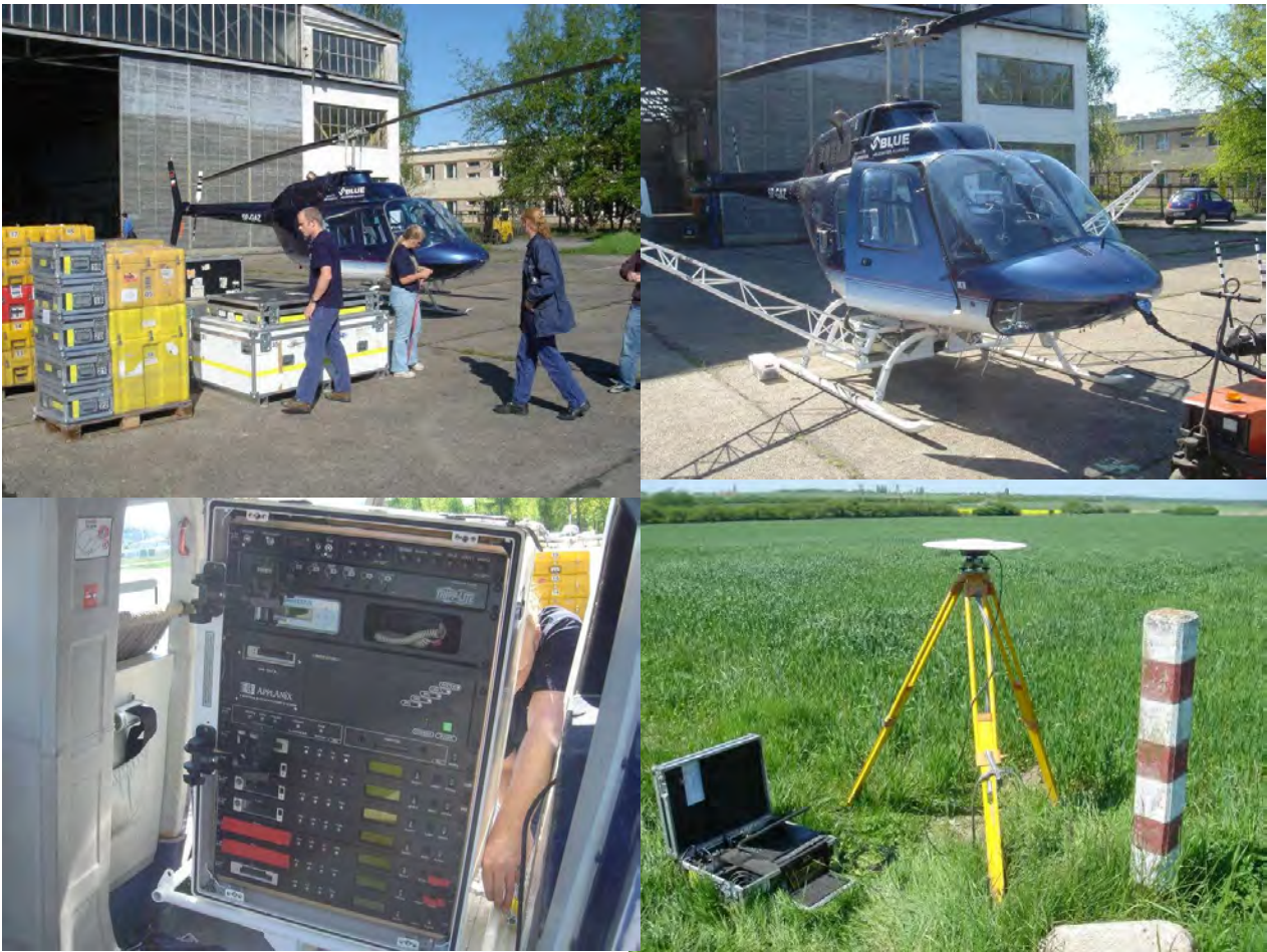
Photos: upper left: FLI-MAP components prepared to assemble on airfield; upper right: system prepared for work; down left: assembling control module on helicopter; down right: ground reference station; Source: Materials of "DEPHOS" and "FUGRO" company
