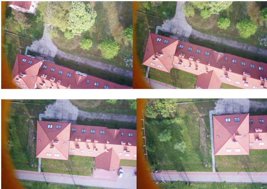
Pic. 3. Exemplary 4 aerial pairs of photos from low-altitude flight approx. 50m (own research).
