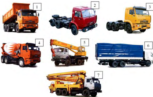
Fig.1 Trucks, special trucks and chassis of KAMAZ: 1 – dump-truck; 2 – chassis for superstructures (add-ins); 3 – tractor; 4 – mixer truck; 5 – crane truck; 6 – board platform truck; 7 – autoconcrete pump
