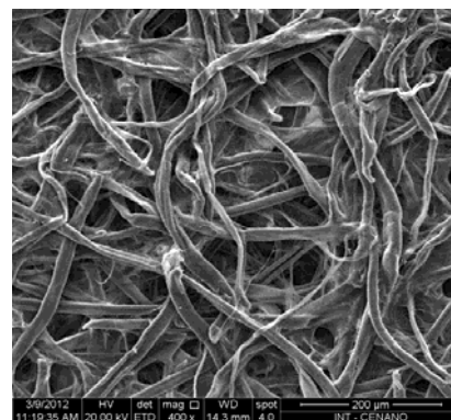
Fig. 2. SEM of a Whatman white paper strip not impregnated with iron-gall ink (magnification of 400x) – blank
