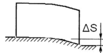
Fig. 4. Vertical dislocations of base under the foundations, which cause the difference of subsidence \Delta S of end walls in the facade plane
