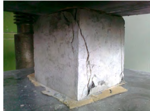
Fig. 5. test cube size 150 * 150 * 150 mm
