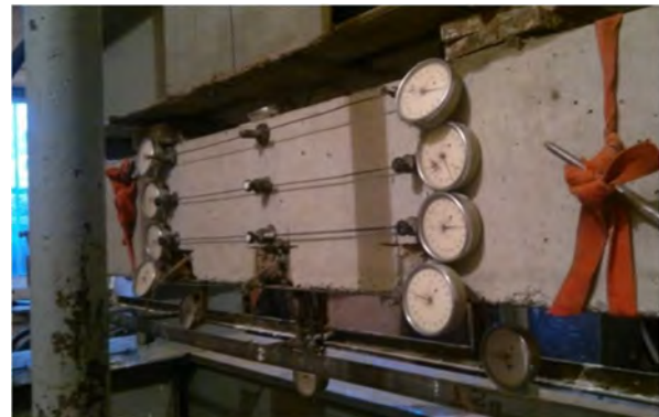
Fig. 7 The test beam. Placing instrumentation.
