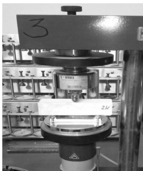
Fig. 1. Determination of flexural strength
