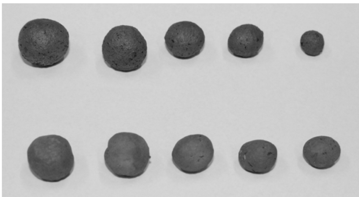
Fig. 2. Images of the obtained lightweight aggregates, calcinated in temperature of 1170°C (CC) – below, (CNaPI) – above
