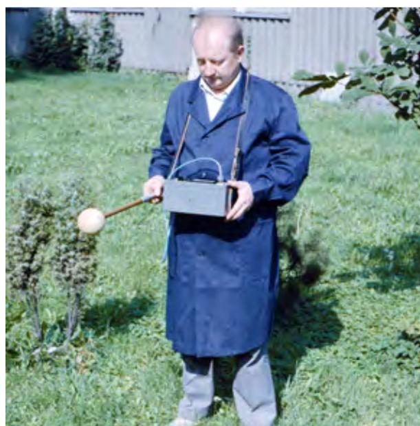
Fig. 4. EMF measurements using an universal EMF meter.
