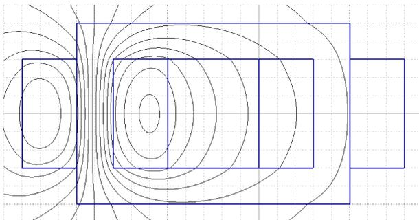
Fig. 4. FEM simulation result representing magnetic field lines located both inside and outside of the investigated sample of magnetic fluid with  $\mu_r = 2$  (planar coordinates).
