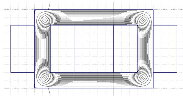
Fig. 3. FEM simulation result representing magnetic field lines in the discussed sample of ferromagnetic material with  $\mu_r = 1000$  (planar coordinates).
