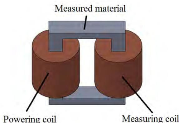
Fig. 2. Principal scheme of classical arrangement for measurement of magnetic permeability of materials.
