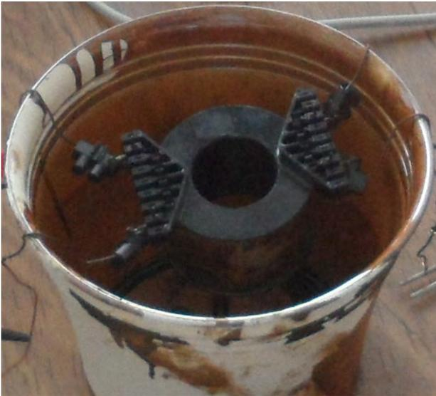
Fig. 7. Measurement transformer without magnetic fluid.
