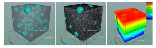
Fig.3. Example of calculating the effective thermal conductivity for composite with spherical inclusions
