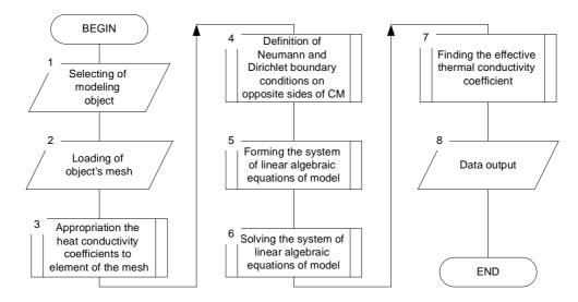
Fig.2. Algorithm for finding the effective thermophysical characteristics of CM
