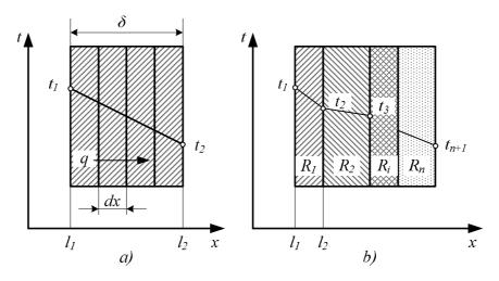
Fig. 1. Model of composite material: a – homogeneous layer; b – multilayered CM
