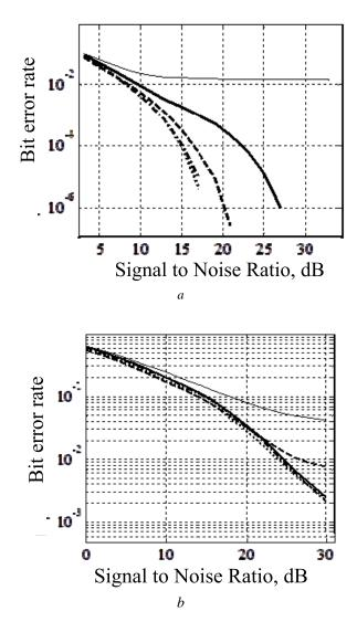
Fig. 5. The dependence of the bit error rate of the signal-noise ratio for different interpolation methods for modulating *a*) QPSK, *b*) QAM16, for channel No. 3
