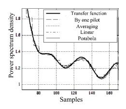
Fig.2 Example of an Assessment of Transfer Function of the Channel by different methods
