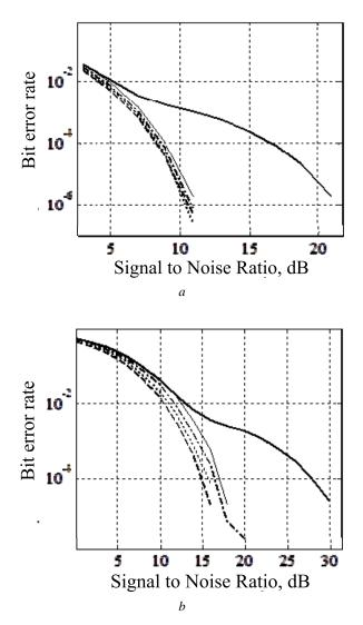
Fig. 4. The dependence of the bit error rate of the signal-noise ratio for different interpolation methods for modulating *a*) QPSK, *b*) QAM16, for channel No. 2
