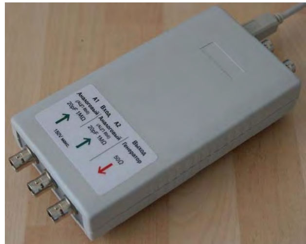
Fig. 6 PV6503 - 4-channel mixed signal oscilloscope. Two analog channels and two digital channels Generator
