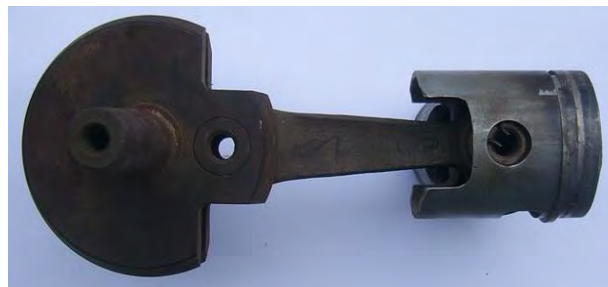
Fig. 1. Real slider-crank mechanism of minibike Jawa 90
