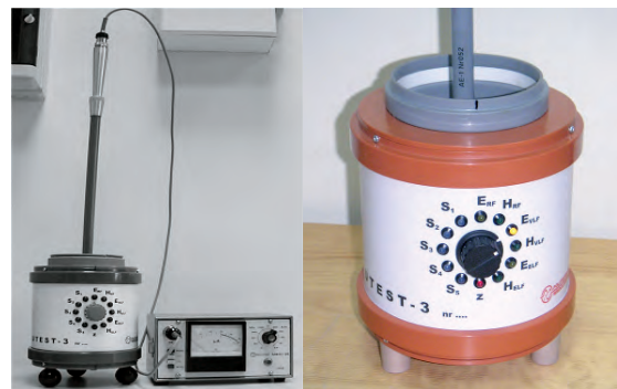
Fig. 4. MEH-type meter tested in UTEST-3 type tester.
