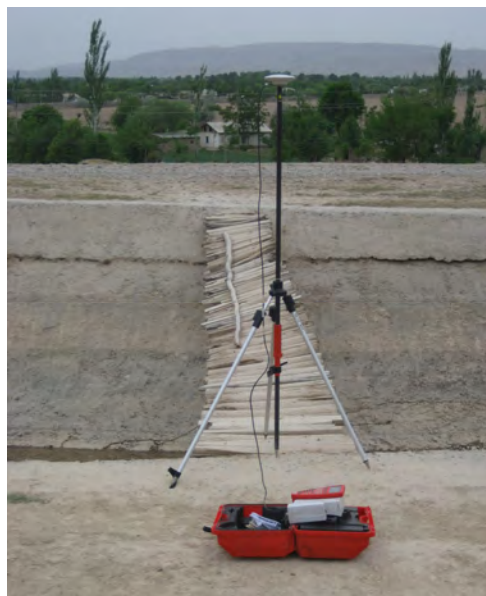
Fig. 2. Measurement of GCP in the field by GPS technique
