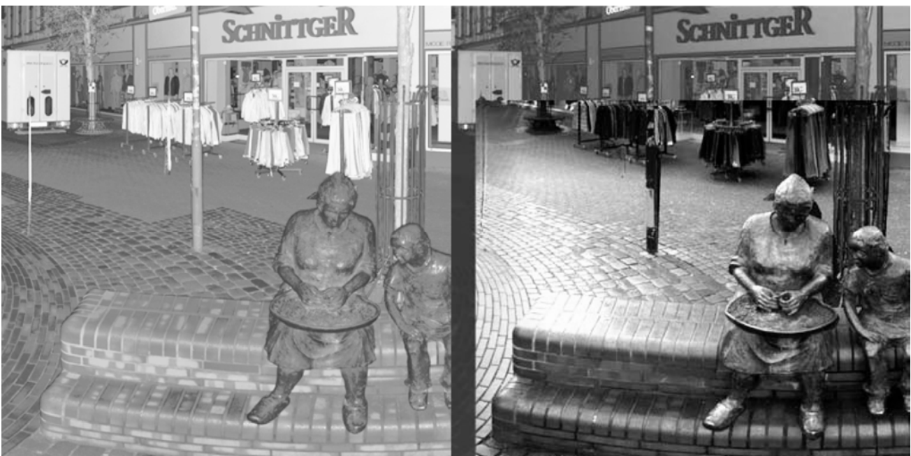
Fig. 5. 3D measurement of a sculpture using laserscanning: a – intensity image; b – superimposition with RGB image
