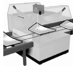
Fig. 8. System for measurement of glass wind shields (Mapvision)
