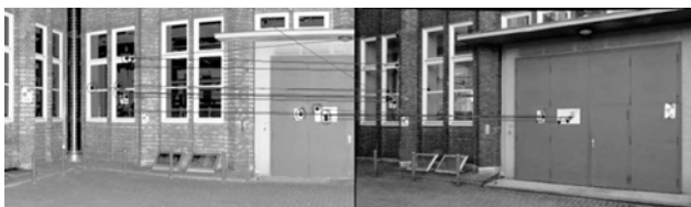
Fig. 11. Matching of interest points in intensity image (laser scan) and RGB image (Shahzad & Wiggenhagen 2010)
