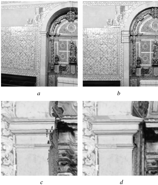
Fig. 10: Orthophoto of a complex building facade (PHOCAD): a – Original image; b – Orthophoto; c – Object modeling using 3D elements; d – Remaining errors of object modeling using a 3D point cloud
