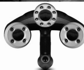
HandyScan 3D: MaxScan Object measurement with photogrammetric tie points
