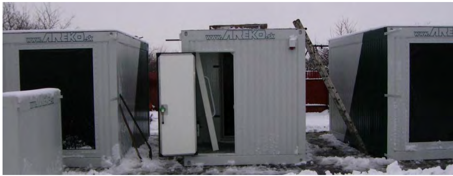
Figure 5. Test boxes- monitoring chambers - view outside
