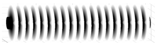
Fig. 17. The change of the dielectric permittivity of a cylinder, modulated by one periodic sequence of rectangular impulses
