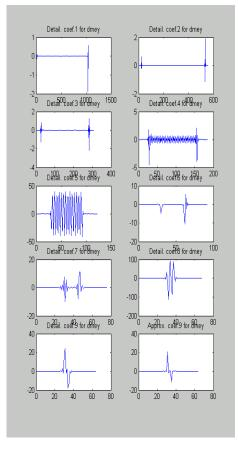
Fig. 1. Graphs of wavelet-coefficients of nine DWT levels of a signal  $\Delta f_{U\Sigma}(t)$  with a low-frequency harmonic component
