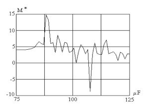
Fig. 1. The dependency of the electromagnetic torque on the capacitance value of the capacitor in the excitation winding
