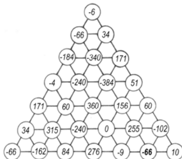
Fig. 6. Difference analogue of biharmonic operator 27/4h^4\nabla^4 for the 20-th node
