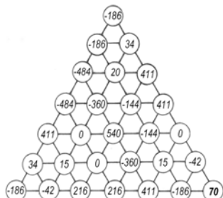
Fig. 7. Difference analogue of biharmonic operator 27/4h^4\nabla^4 for the 26-th node
