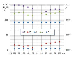
Fig. 1. Dependence of the parameters of SC on the current and the heat losses in the diffusion layer
