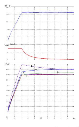
Fig. 2. Time-response characteristics  $U_{bat}(t)$ ,  $I_{ch/dch}(t)$ ,  $U_{sc_i}(t)$ in the charge mode of the battery by a relay current regulator (Here and throughout: 1 – SC with nominal parameters, 2 – C-10%, 3 – R+10%, 4 – B-50%, 5 –  $\mu$ -20%)
