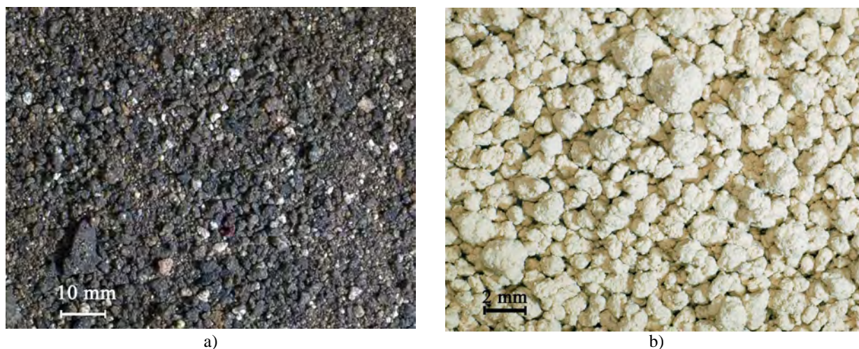
Fig. 1. Appearance of native (a) and saponite mineral activated by hydrochloric acid (b)
