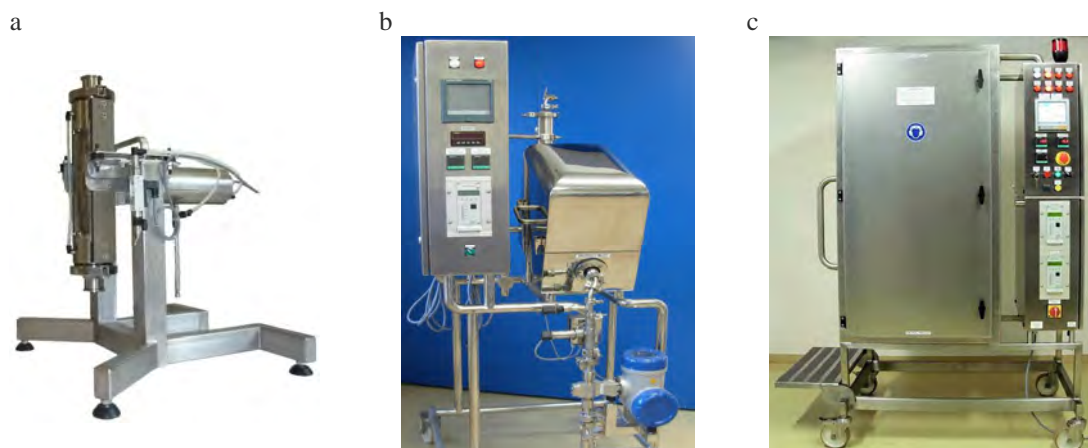
Figure 2: Example of SONITUBE ® realisation : 20kHz basic (a), 35kHz instrumented for pharmaceutical industry (Sene et al., 2012) (b) and 20kHz instrumented for industry (c)
