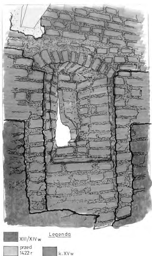
Fig. 13. Crenellation conversions, compiled by W. Niewalda; grey color – 13/14th century; pink color – before 1422, blue color – loop hole, 1490 s.
