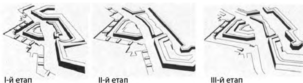
Fig. 3. The Vauban's three bastion system
