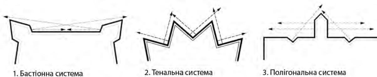
Fig. 4. Three tracings of defensive systems: bastion, tenail and polygonal
