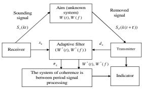
Fig 1. Structure of adaptive channel of treatment of radiolocation signals
