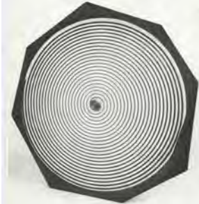
Fig.1. Disk metal-dielectric structure with spiral nonuniformity
