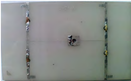
Fig.1. Plate of power limiter of S-band with microstrip elements made from photopolymerized paste 1785 on poli-coat substrate.
