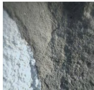
Fig. 3. Optical microscopy for the splinter of the expansive composition hardened seven days under compressed conditions
